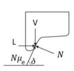
$$\frac{L}{V} = \frac{(Normal\ Force) \times sin(\delta) - (Friction\ Force) \times cos(\delta)}{(Normal\ Force) \times cos(\delta) + (Friction\ Force) \times sin(\delta)}$$
