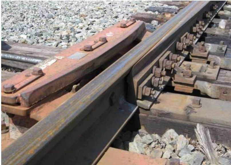
Western Cullen Hayes has an adjustable and replaceable wear bar
