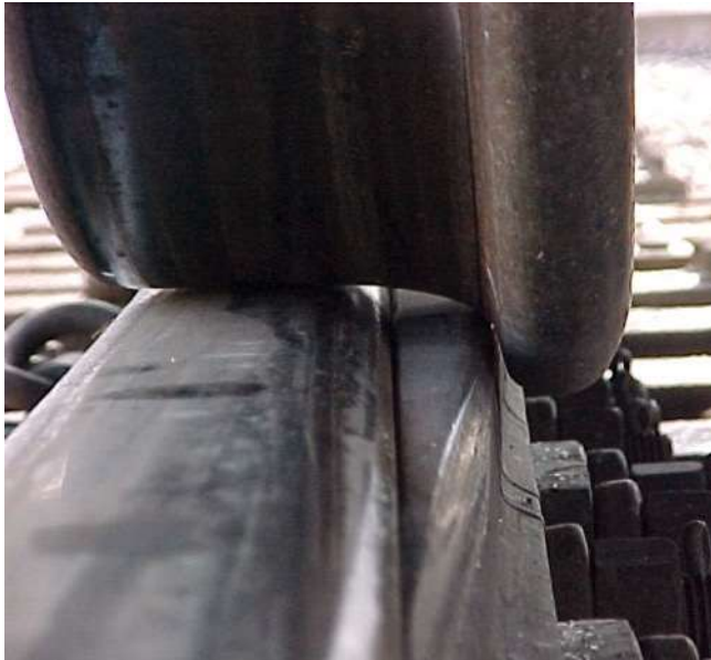
Switch point below stock rail
