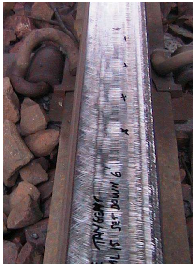
Grinding stone chatter (pressure control)
