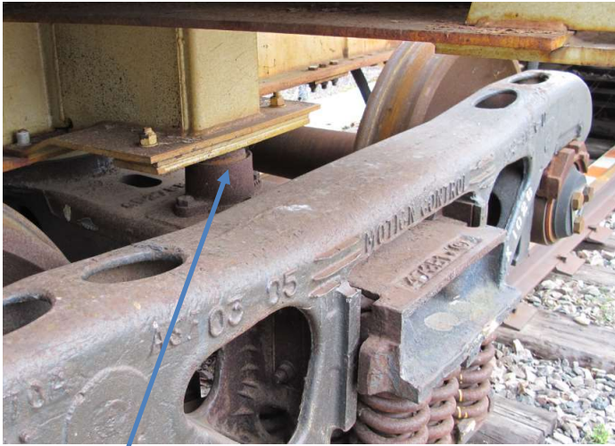
Constant contact side bearing
