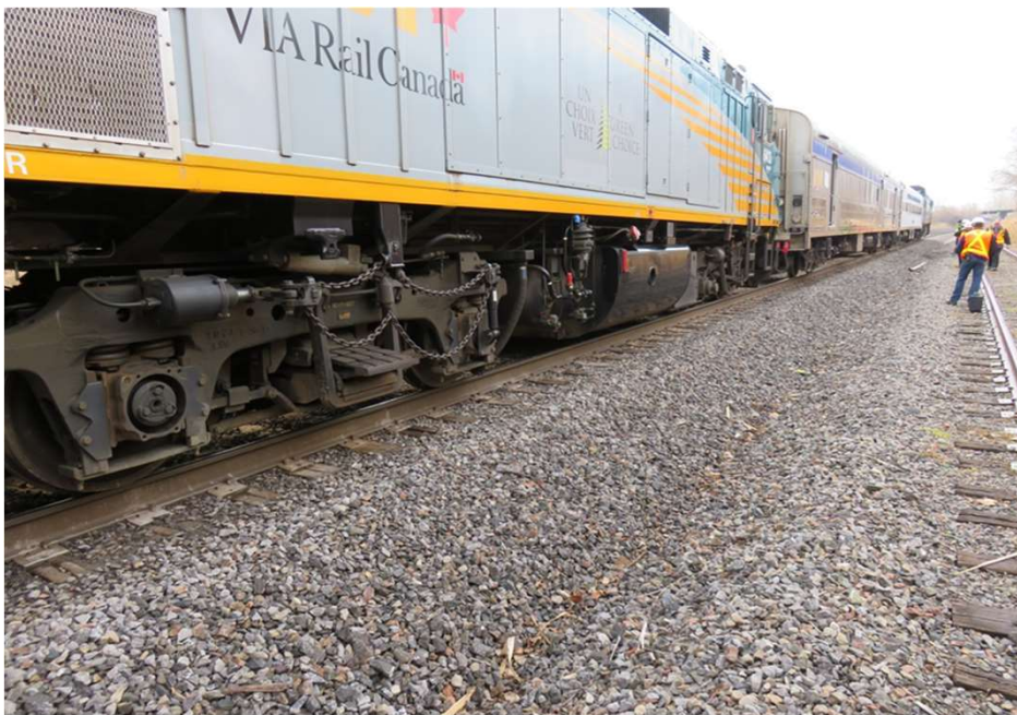
Front Truck of Middle Locomotive Derailed to Left
