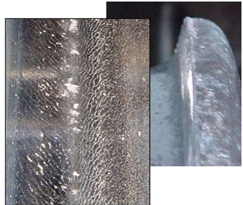
Flange wear and wheel damage
