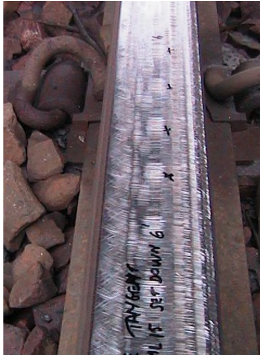
Grinding stone chatter (pressure control)
