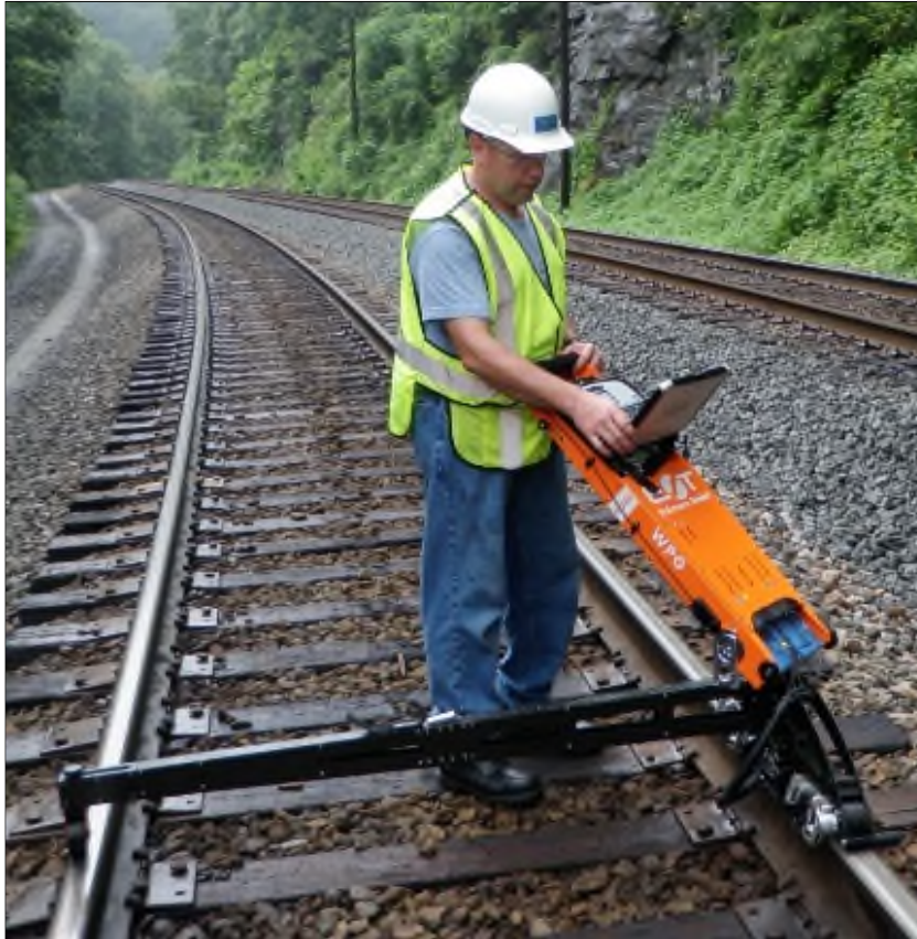
Rohmann Draisine (eddy current)
