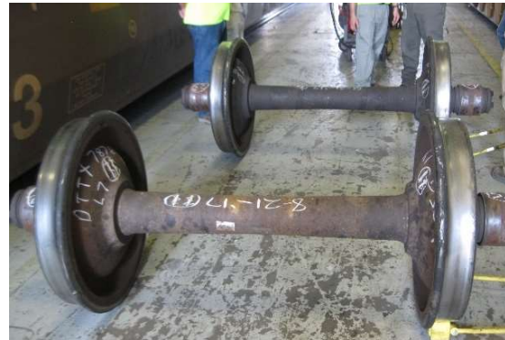
These wheels show some flange contact with the ground, but not enough to have been the first to derail (they would have run over 2 turnouts and a diamond).
