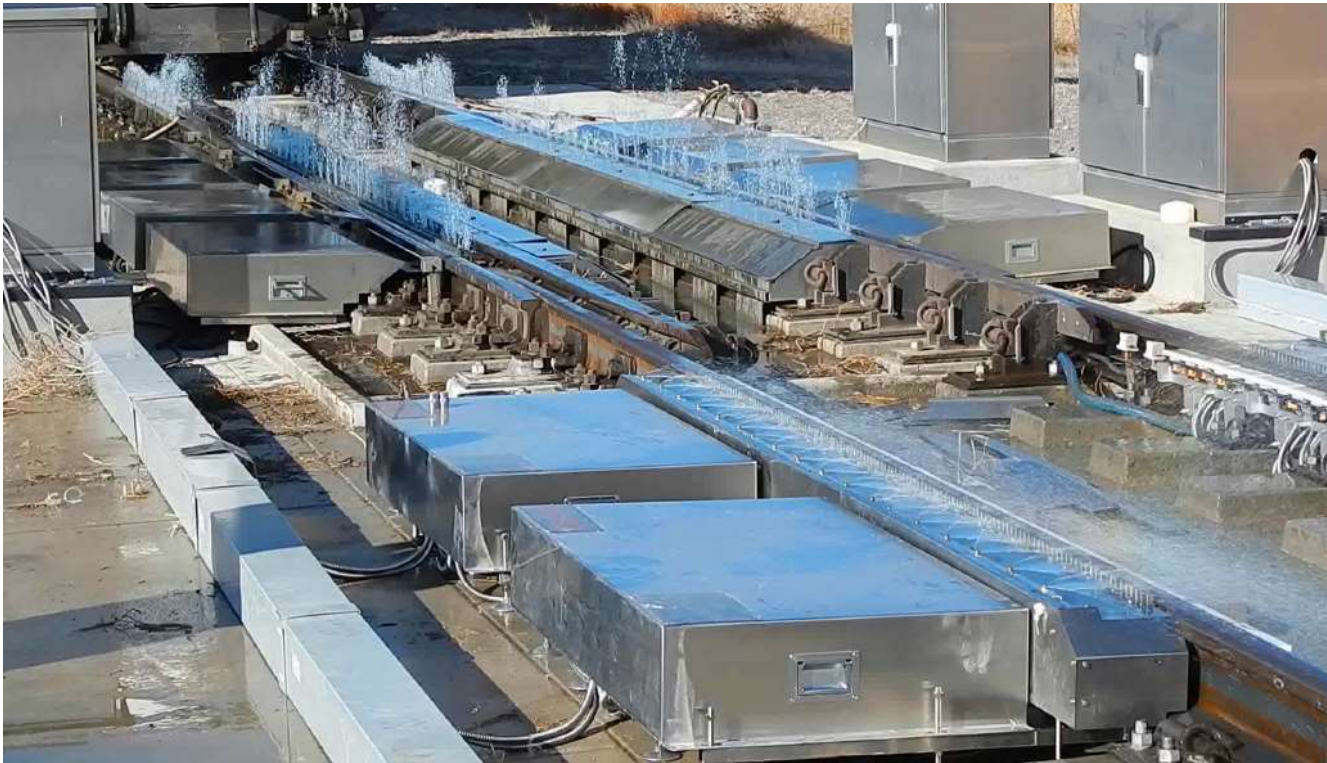
Image from Proceedings of 2018 AAR Review Matthew Witte, "Effectiveness of Cracked Rim Detectors to Identify Broken Wheels"
