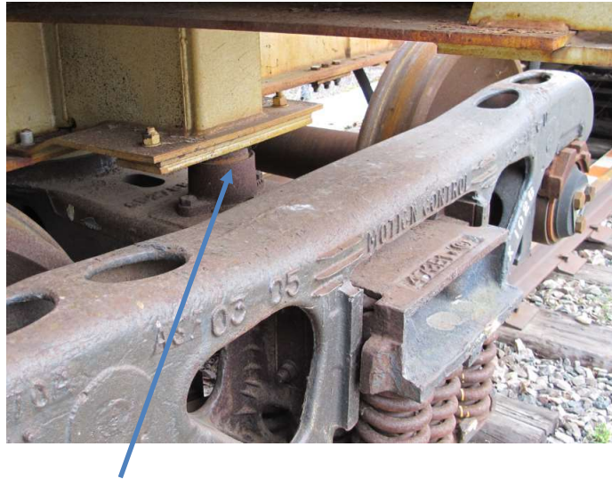
Constant contact side bearing
